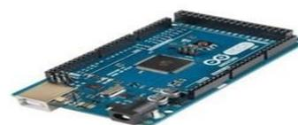
Gambar 5 Arduino Mega 2560
