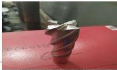
Gambar 3.4 Endmill HSS Ø20 mm
