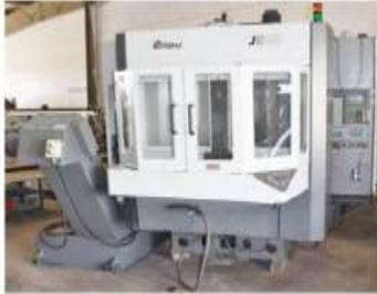
Gambar 3.3 Mesin CNC milling
