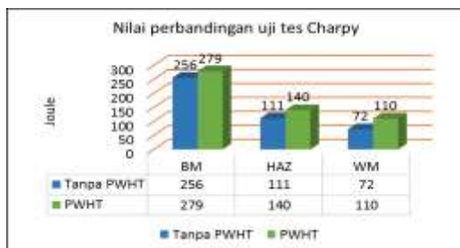
Gambar 21. Diagram Hasil Perbandingan Impact Metode Charpy
