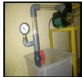
Gambar 12 Pemasangan *ball valve*, *pressure gauge* dan *vacuum gauge*.
