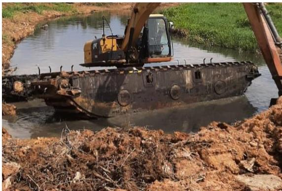
Gambar 4. Ponton Excavator Amphibious
