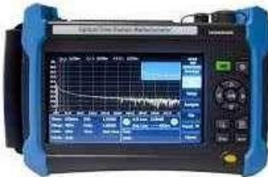
OTDR Fiber Optic (<https://it.telkomuniversity.ac.id/alat-ukur-fiber-optik-otdr-dan-opm/>)
