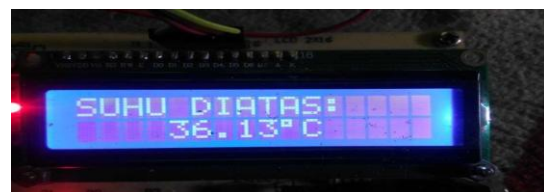
Gambar 7. Tampilan LCD 16 x 2
